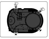
If lifting with a crane, use lifting straps!
